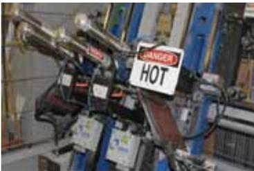
**PVC Window Manufacture** - The manufacture of PVC Windows generally involves sections of PVC frame material which are heated and welded together to form the finished window frame. PTFE glass tape or fabric, applied to the weld plates, allows rapid heat transfer from the heat plate to the PVC sections, while preventing melted PVC from sticking to the plate surface. This results in a clean weld, a clean surface on the weld plate, and faster, uninterrupted window production.
