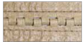
PTFE/Glass Fabric edges are heat-sealed on a mesh dryer belt.
