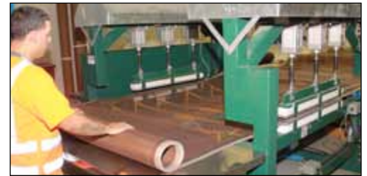
PTFE/Glass Fabric edges are heat-sealed on a mesh dryer belt.
