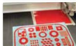
**Engineered Nested Kits** - For complex and repetitive masking of an identical set of parts, custom kits of precision pre-cut shapes save considerable time and cost. Multi-profile templates are generated from customer supplied specifications or CAD drawings.
