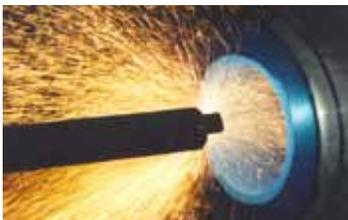
**Arc Spray** - The primary challenge associated with the Arc Spray coating process is the wide spray plume that exits the gun. This results in the necessity of primary masking, close to the target zone, and secondary masking to protect large non-target areas from overspray and costly clean-up or re-work. While arc spray is not as abrasive as other spray processes, it still requires proper masking to ensure protection of the part and non-target surfaces.
